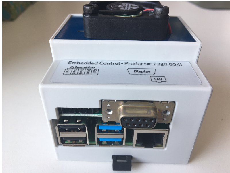
Figure 13: LAN and display port. The USB ports remain unused.
