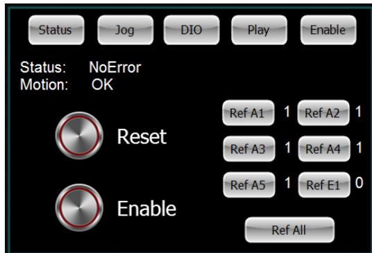
Figure 44: To do this, press the "Play" key at the top of the display and use the "prev" and "next" keys to select a program written for your robot.
