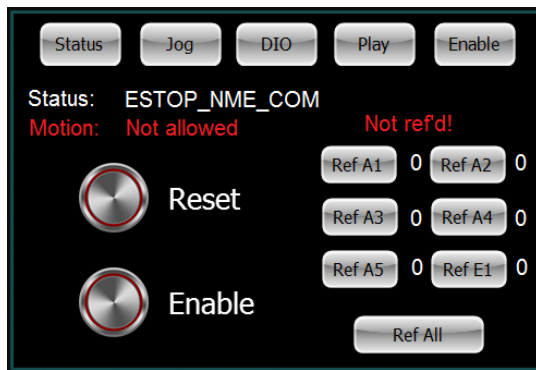
Figure 38: Press the "Enable" button in the top menu (top right) on the touchscreen display to go to the Enable page.
