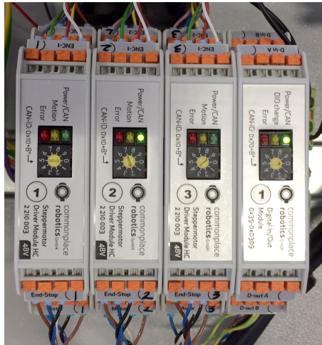
Figure 2: Three motor modules with 4 connectors per module, each leading to a motor and the corresponding reference sensor. Also in the picture: a digital I/O module (module on the right), which is not wired.
