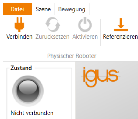
Figure 17: Buttons for connecting to the hardware, resetting errors and activating the motors, referencing and "Status" display.
