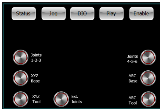
Figure 41: To do this, press the "Jog" key at the top of the display. 2. Press "Joints 1-2-3". Then move and rotate the joystick. You can now move axes 1, 2 and 3. 3. Press "Joints 4-5-6". Now move axes 4 and 5 by moving and turning the joystick.
