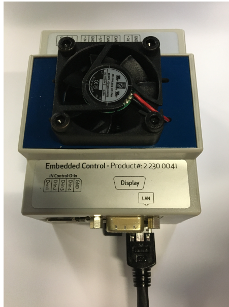
Figure 3: Integrated control computer with LAN cable.
