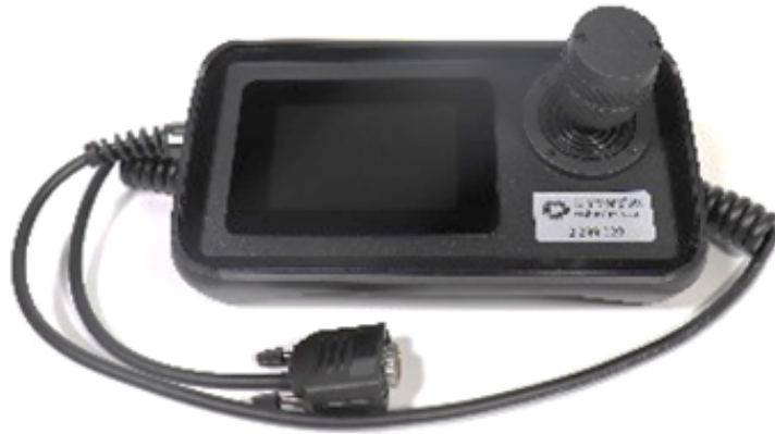
Figure 14: Handheld control unit (touch display and 3-axis joystick)
